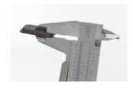
First check the brake pad width visually. If you suspect that the minimum width is exceeded, the pads must be dismounted and inspected with a calliper. Please consult a specialist workplace for this inspection.
