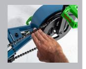
During maintenance works a trapping and crushing risk exists. Your fingers can get caught by moving parts.
