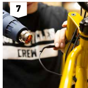
7 Pull the shrinking tube over the plug connection and heat it up with approx. 300 degrees .
